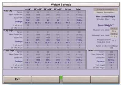
The page shows the amount of weight savings, highlighted in blue, using SmartWeight<sup>®</sup> balancing technology. The savings are shown in both actual weight and percentage.
