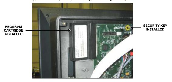
Install the supplied electronic security key in the button socket on the board within the support assembly.
