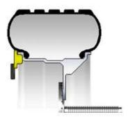
Measure the distance from the left weight plane to the desired right weight plane, using a tape measure. This distance must be in millimeters (convert inches to millimeters by multiplying by 25.4). Measure the weight plane diameter manually, using caliper or tape measure.
